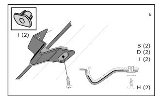
6. Re-fit the hood protector centrally to hood. Secure the hood protector with center metal clips to hood screw plug and self drilling screws provided. **Note:** Ensure the clips fit tightly against the hood lip. If necessary detach the hood protector from the clips and re-align clips tightly to hood.
