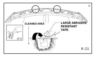
3. Clean center metal clips locations with alcohol wipe provided. Wipe off any residue with a dry clean cloth. Adhere the large abrasive resistant tape strips over the hood lip. Apply tape so approximately half of each strip is adhered to the topside and half is adhered to the underside of hood.
