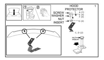
1. Clean installation area thoroughly and open the hood. Position the nut inserts into the center metal clips and metal wing clips, as shown. Secure **center** metal clips to hood protector with a small screws and washers. Center screws on part covering slots.
