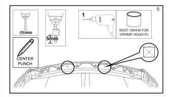
5. Find the center of the square hole on the masking tape by joining the corners of the square (see image). Center punch then drill Ø6mm holes at the center of the square holes. Remove any metal shavings and remove masking tape from hood. Apply rust inhibitor (999MP-9G001P) around the raw edges of the drilled holes.
