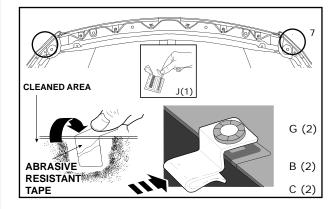
7. Clean the noted areas under the wing clip locations with alcohol wipe provided. Wipe off any residue with a dry clean cloth. Adhere the abrasive resistant tape strips over the hood lip. Apply tape so approximately half of each strip is adhered to the topside and half is adhered to the underside of hood. Locate the outer metal wing clips over the abrasive resistant tape strips on the hood lip.
