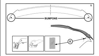
9. Clean the two bumpon areas (bumpon positions) with alcohol wipe provided. Adhere the small abrasive resistant tape strips over hood lip. Apply small abrasive resistant tape to the top surface of hood directly under where bumpons are installed on product.
