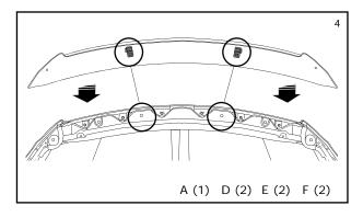
4. Re-fit hood protector to hood. Apply masking tape to hood underneath the square holes in the center metal clips. Mark the outline of the square hole onto the masking tape. Remove the hood protector.
