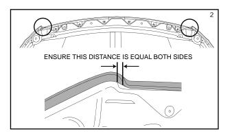
2. Trial fit hood protector on hood. Align the hood protector in the center of the hood by ensuring the distance between the edge of the hood and hood protector is equal on both sides (in the area shown). Mark location where the abrasive resistant tape should be applied (two center locations).
